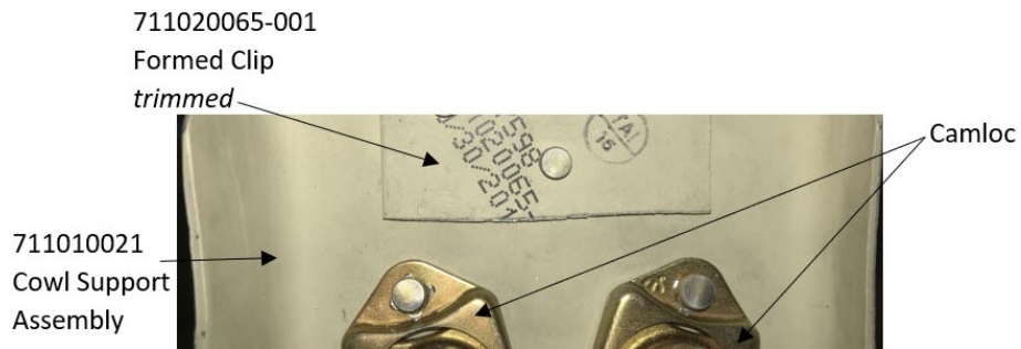
Figure 8-15 Inboard Side of Cowl Support Assembly *Formed Clip & Camloc already installed for Edge Distance Reference*
